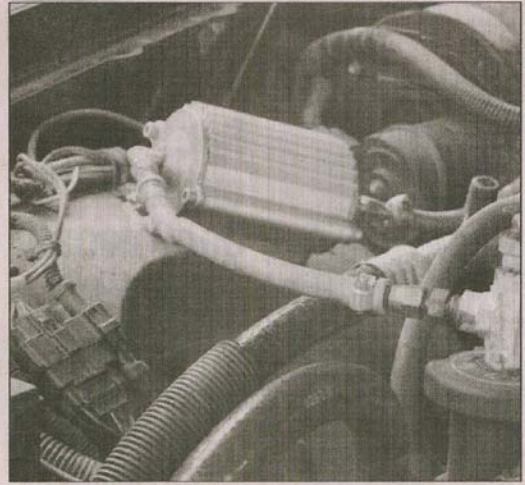
The NTZ Micro Filtration device installed on a Hillsdale County Sheriff's Department patrol car. The supplemental filter has more than doubled oil life in the test vehicle.
