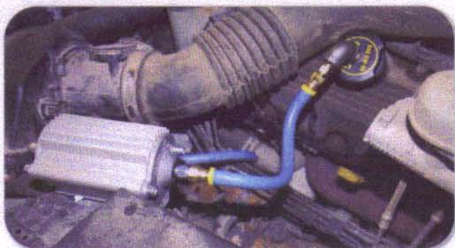
An NTZ filter installed on the Hillsdale County, MI Sheriff's Ford CVPI.
