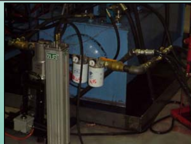
Test Stand Sump & example of the contamination the NTZ Filter captures.
